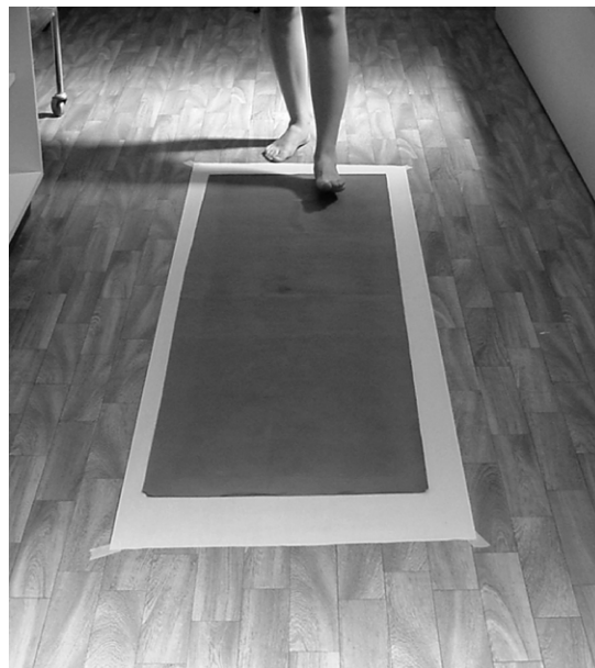
Figure 1. Procedure used to obtain the footprint to measure the angle of gait.
