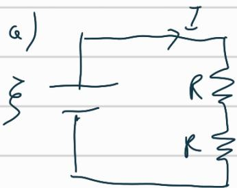
$$P = \xi I \quad \text{Calculando } I \text{ usando } R \text{ y } V$$
