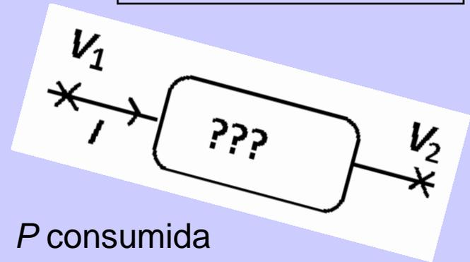
$$P = I(V_1 - V_2)$$
