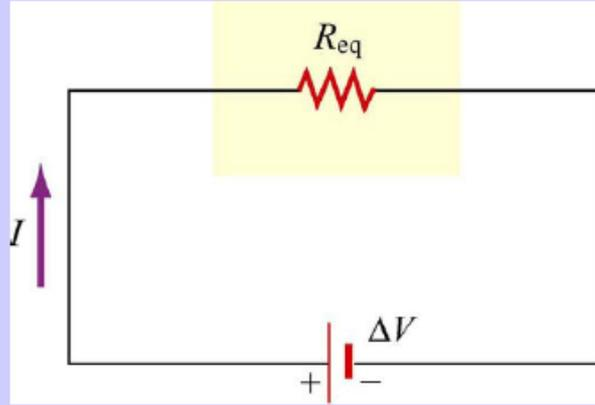
$$\Delta V = \Delta V_1 = \Delta V_2 \Rightarrow \Delta V = I_1 R_1 = I_2 R_2 = I R_{\text{eq}}$$
