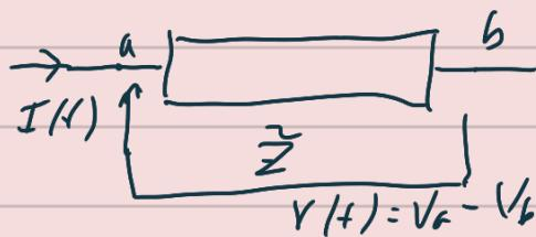
$$P(t) = V(t) I(t) \quad \text{con} \quad \begin{cases} V(t) = V_0 \cos(\omega t) \\ I(t) = I_0 \cos(\omega t + \phi_{IV}) \end{cases}$$
