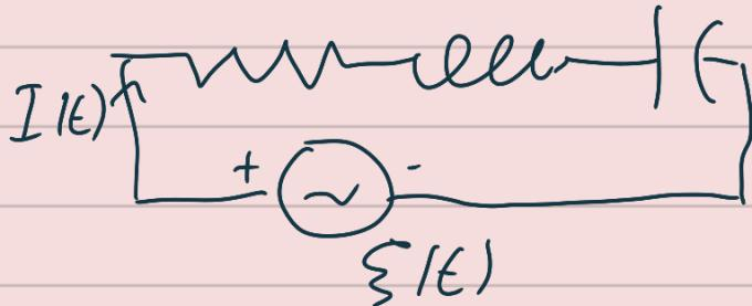
$$\text{Con } \tilde{Z}(t) = \tilde{\Sigma}_0 \cos(\omega t) \\ I(t) = I_0 \cos(\omega t - \varphi_2)$$
