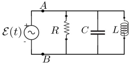
$$\xi(t) = 216 \cos(2000t) \text{ V} \Rightarrow \tilde{\xi} = 216 \text{ V. } R = 180\Omega; \tilde{Z}_C = -40j\Omega, \tilde{Z}_L = 120j\Omega$$
